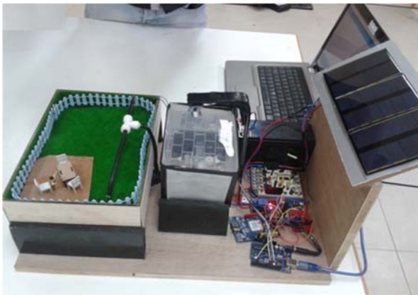
Fig. 5. The laboratory-developed prototype of fully automated irrigation system.
