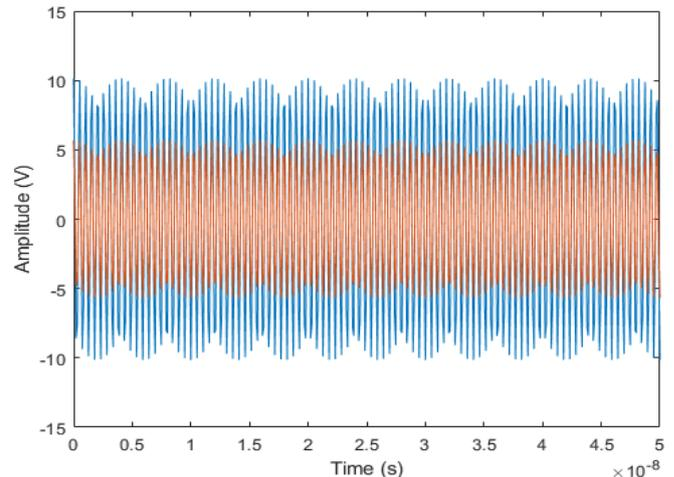
**Figure 4.** IFC Signal Modulated on Carrier Frequency
