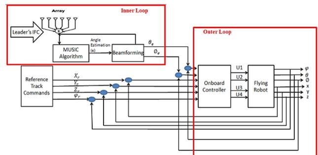
**Figure 3.** Flying Robot Control System
