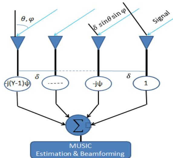
**Figure 2.** Array of Antenna configuration and phase estimation
