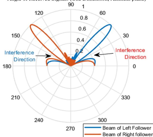
**Figure 8.** The Beamforming Response Main Loops directed to Leader Angle ( $45^{\circ}$ ,  $135^{\circ}$ ) for Left and Right Follower respectively, the Direction of Interferences are Ignored with Null (Zero Power)
