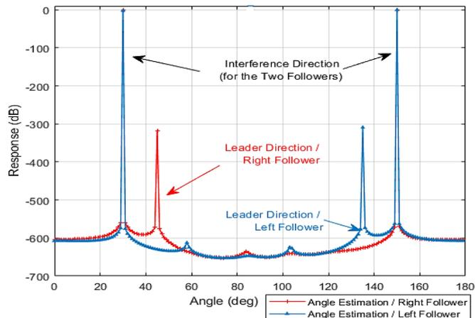
**Figure 7b.** The Response of Music Algorithm for Estimation the Angle of Received Signals (One Dimension, Azimuth plane)
