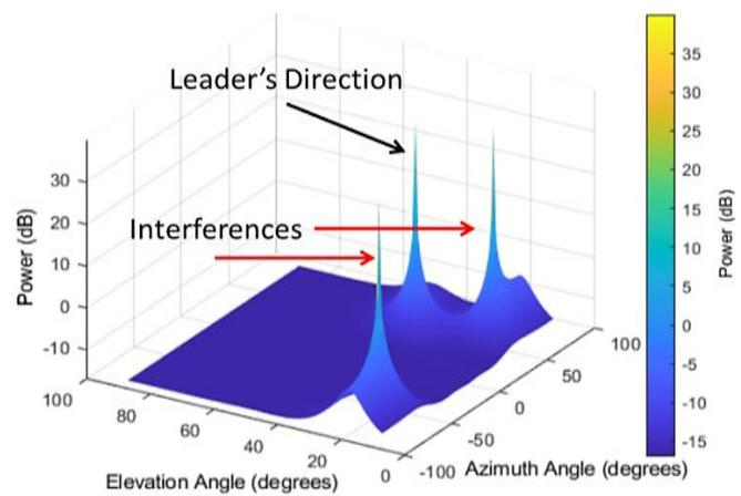
**Figure 7a.** The Response of Music Algorithm (Three Dimensions, Azimuth and Elevation)
