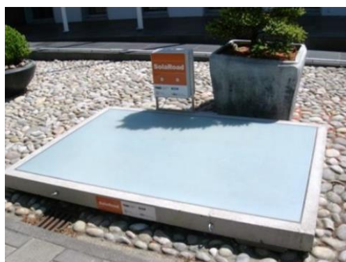
Figure 13. Solar Road prototype panel
